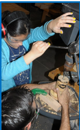
Feliz using a drill press to make a hole for the pen holder.
