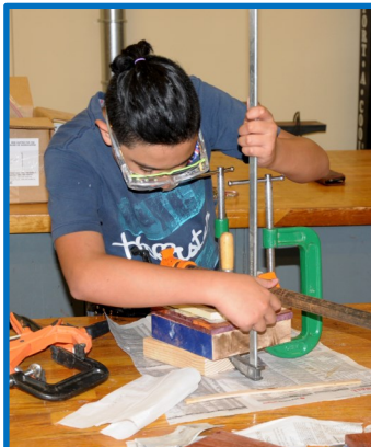
Pedro placing clamps on his wood project so the glue can dry properly.
