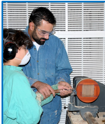
Alex using a hand tool to round the corners on the lathe.
